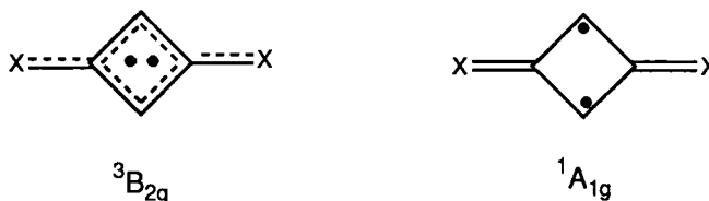
Figure 9 Bonding in the lowest electronic states of DMCBD ( X = CH_2 ) and in CBDOD ( X = O ).
